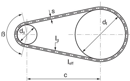
$$l_{eff} = 2c \cdot \sin\left(\frac{\beta}{2}\right) + \frac{\pi}{2} \left[ d_s + d_l + 2s + \frac{(d_l - d_s)(180 - \beta)}{180} \right] \text{ [mm]}$$
